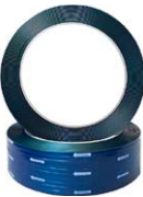
PETH92065406 PET Green Strapping Embossed 9.2mm x 0.65mm x 3000m Core: 406mm Break Strain: 189kg ±10%
